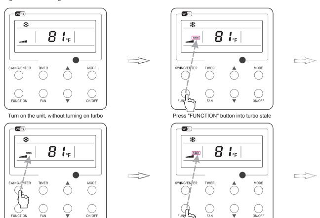
Press "SWING/ENTER" button to turn on turbo function
