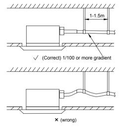
The incline of attached drain hose should be 75mm or less so that the drain outlet does not have to withstand additional force.
