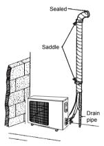
If the outdoor unit is installed higher than the indoor unit.
