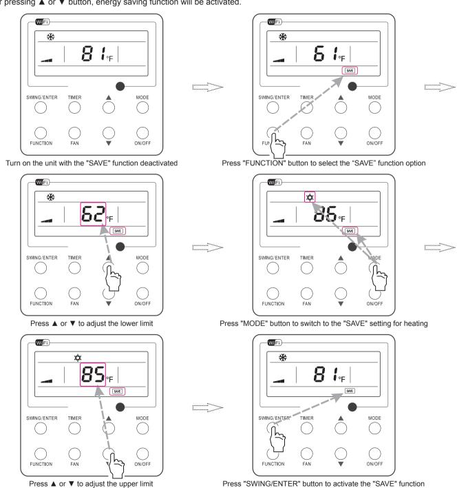
Fig. 13 Energy Saving Function Setting
