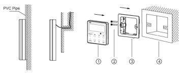
Fig. 22 Accessories for the Installation of the Wired Controller
