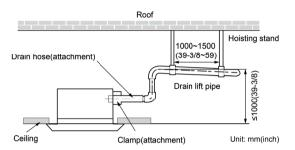
Secure a downward gradient of 1/100 or more for the drain pipe. To accomplish this, mount supporting brackets at an interval of 1-1.5 m.
