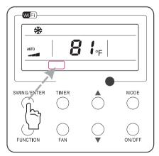
Press "SWING/ENTER" button to turn off X-fan function
