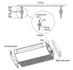
(6). Reinstall and tighten the right and left side panel.
